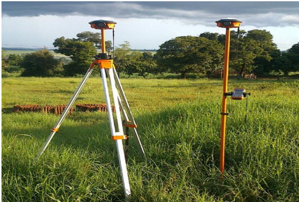
Figura 1 – Receptores GNSS/RTK Navcon SF 3040.
