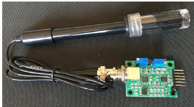
Figura 17: Sensor pH E-201.
